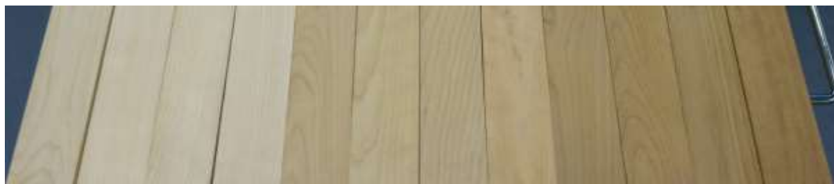
Figure 2. Sawn birch wood material, thermally modified at 170 °C (left), 185 °C (middle), and 200 °C (right).
