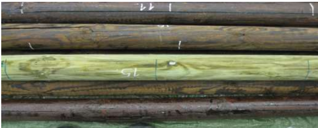
Figure 3. Brown-coloured, pine oil impregnated fencing posts. The green reference is impregnated with copper-based preservative.
