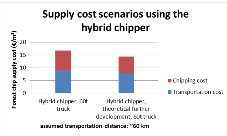
**Figure 3.** Average total forest chip supply costs for two chipping scenario cases applying the hybrid chipper for a one-year supply of logging residue chips to an example CHP plant.
