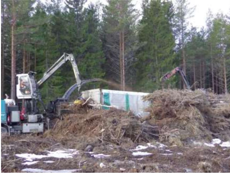
**Figure 2.** Hybrid chipper when chipping logging residues and blowing them onto a truck-trailer transportation vehicle.
