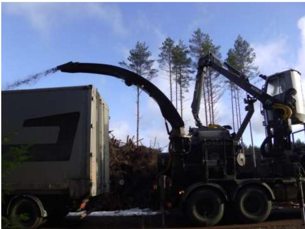
**Figure 1.** Hybrid chipper when chipping logging residues at a roadside site.
