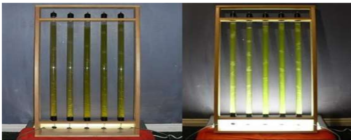
Figure 3. Micro Algae Tubes for CO 2 capture and utilisation. 3
