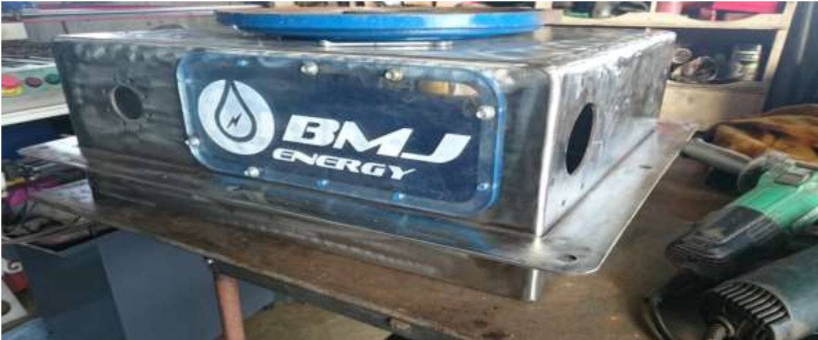
Figure 4 The box which drives the water from stream into the pipes 4
