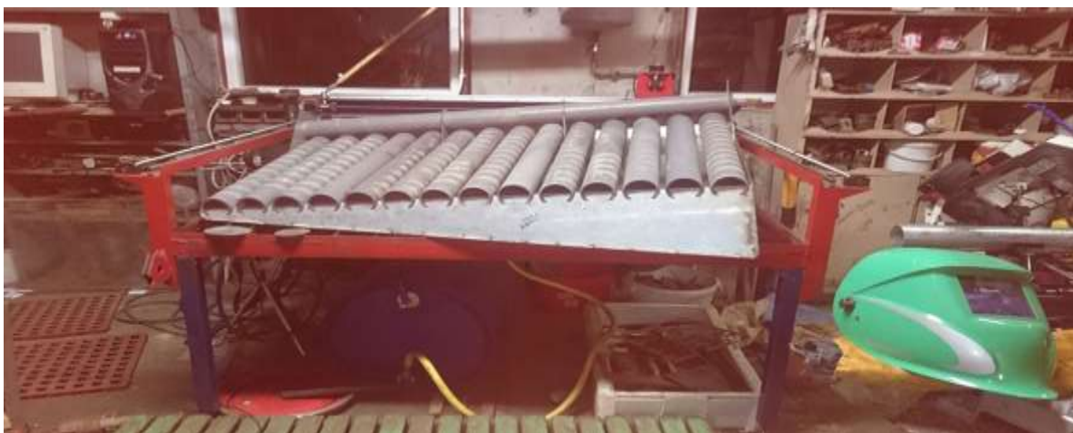
Figure 3. The box which should filter mud and sand more efficiently than before. 3
