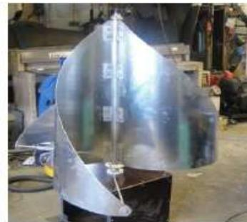
In 2010, the turbine got bigger and now made from aluminium and steel. Fixed with a generator and installed on a cabin.
