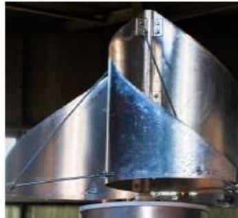
In 2013, the focus was on optimizing choice of materials and stainless steel selected to minimize corrosion. Stainless steel bearings were added and experimented with custom-made generator.
