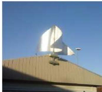
In 2009, the first IceWind wind turbine concept was built with fibreglass and tested without a load. The quality of low start-up speed was discovered.
