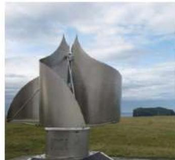
In 2014, the first 1000W turbine built and installed on IceWind HQ for stress tests. The turbine got weight reduction as well as strengthening with carbon fibre.
